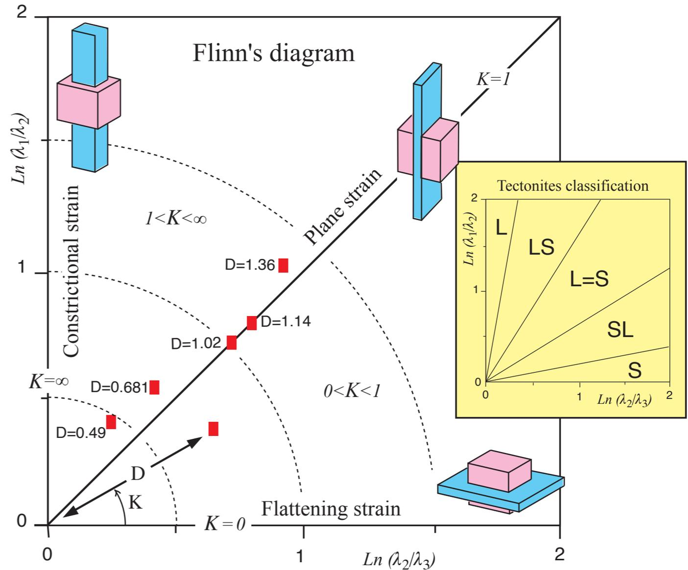
Strain-related fabric depend on the shape of the finite strain ellipsoid. Pancake shaped ellipsoids lead to *S tectonites* (strong schistosity, no lineation), cigar shaped ellipsoids lead to *L tectonites* (strong lineation, no schistosity). *L=S tectonites* are produced by plane strain.
