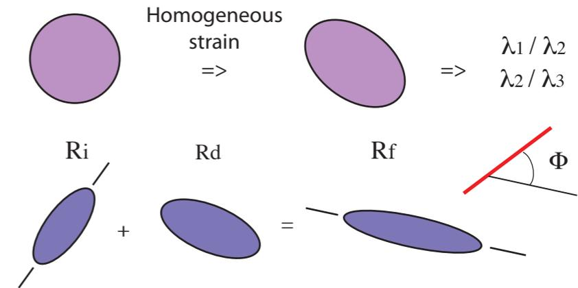
$$R_d^2 = R_{fmax} \cdot R_{fmin}$$
