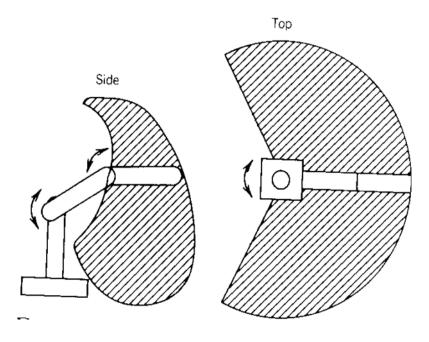
Fig.11: Articulated robot with workspace (a) Side view (b) Top view.
