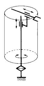
Fig.5: Workspace of Cylindrical Coordinate Robot.
