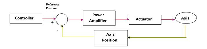
**Fig.13: Control loop of a servo-controlled robot**
