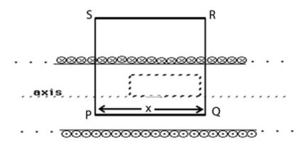
A solenoid is a ling cylindrical coil having number of circular turns. Consider a solenoid having radius R consists of n number of turns per unit length. Let P be the point at a distance x from the
