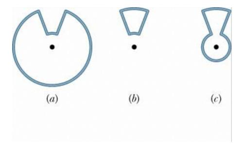
**Note on problems** when you have to evaluate a B field at a point from several partial loops Only loop parts contribute, proportional to angle (previous slide)
