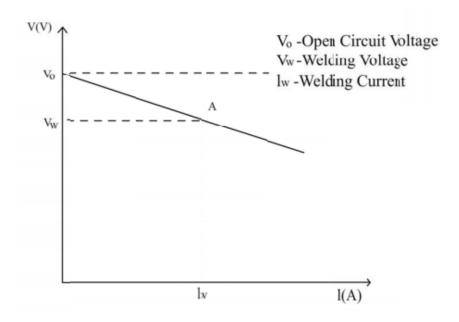
Fig. 3.2 Static characteristics of constant voltage welding power source
