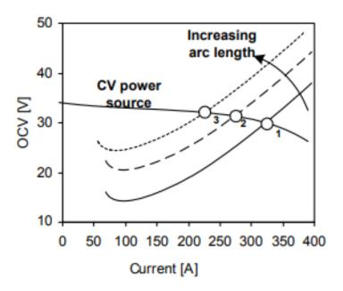
Fig. 3.3 Static characteristics of constant voltage welding power showing operating points with increasing arc length
