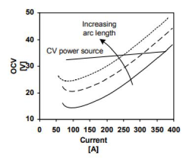
Fig. 3.4 Static characteristics of rising voltage welding power showing operating points with different arc length
