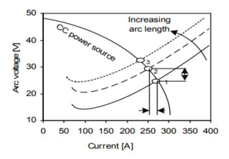
Fig. 3.1 Static characteristics of constant current welding power source
