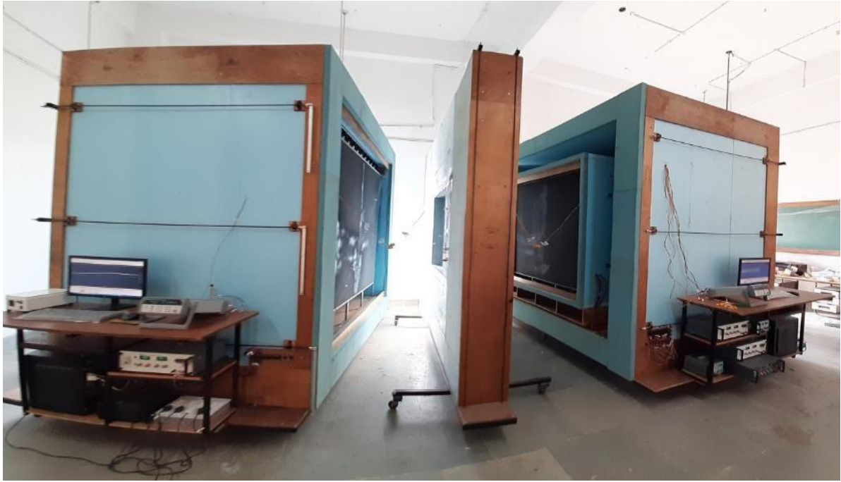
Guarded Hot Box Test Facility Designed & Developed for U-Value measurement
