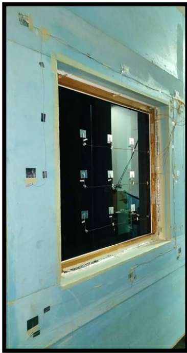
Guarded Hot Box Test Facility Designed & Developed for U-Value measurement
