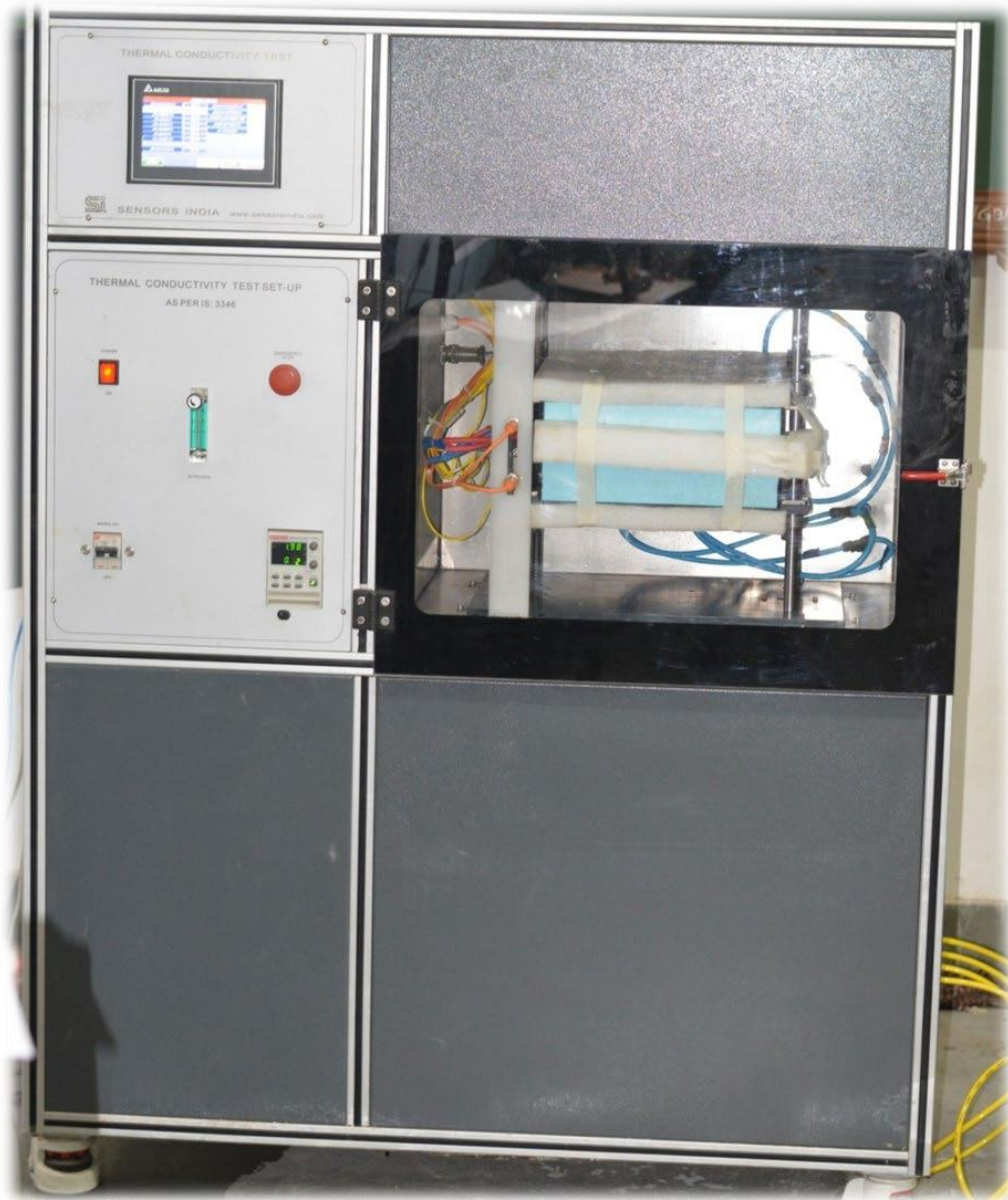
Thermal conductivity Measuring Setup
