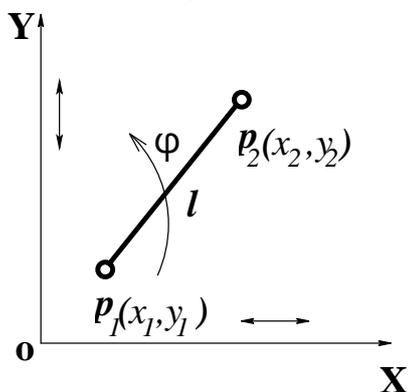
Figure 3: A rigid link in planar motion
