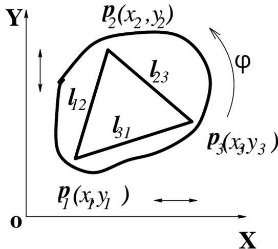
Figure 2: Rigid body in planar motion with three-degrees-of-freedom
