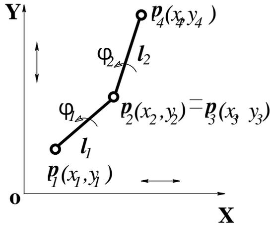
Figure 5: Two planar links with a rotary joint
