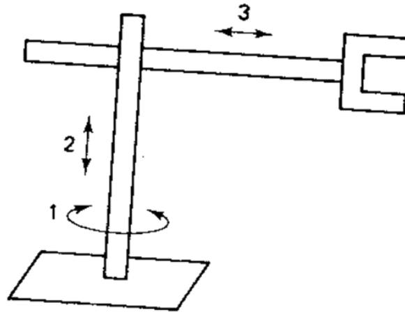
**Fig.4: Cylindrical Coordinate robot**
