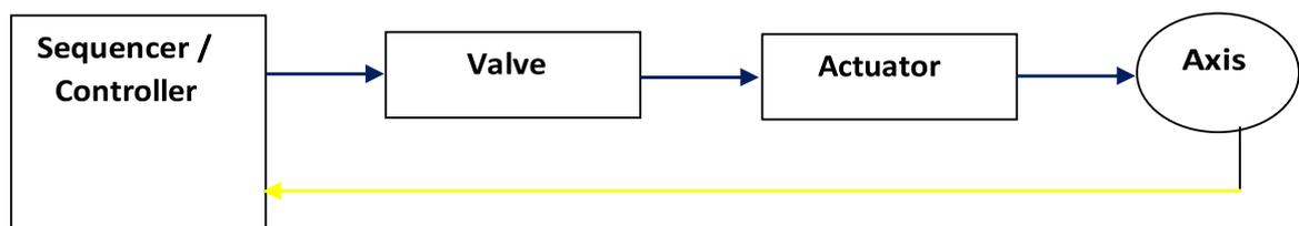
**Fig.12: Control loop for a non-servo robot**
