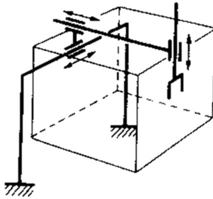
**Fig.2: Workspace of a cartesian coordinate robot.**
