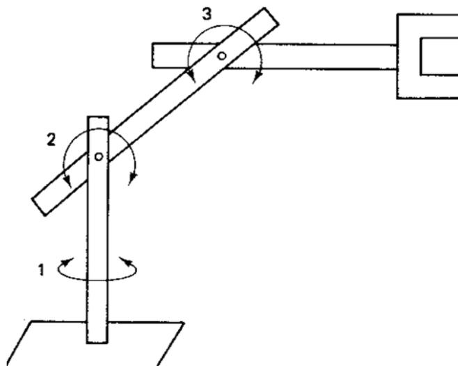
**Fig.10: Articulated coordinate robot**
