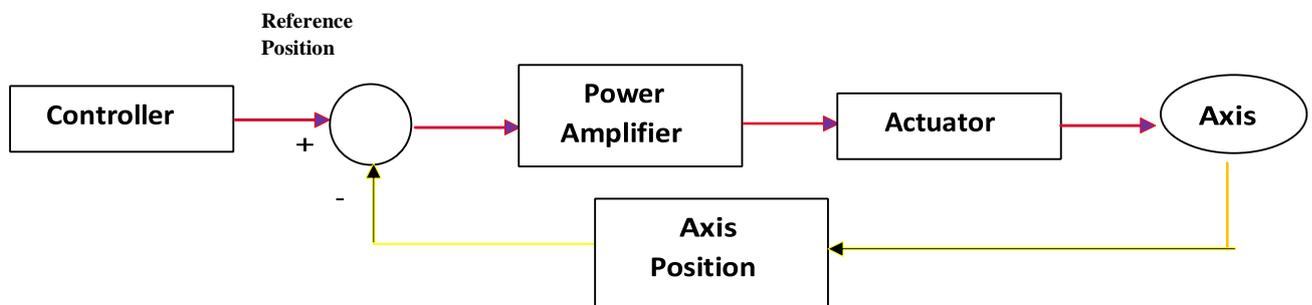
**Fig.13: Control loop of a servo-controlled robot**
