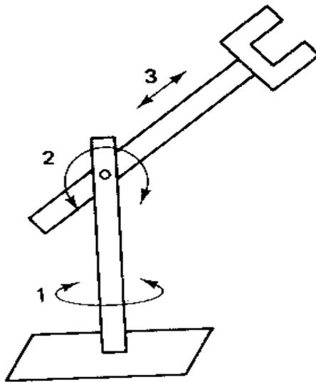
**Fig.7: Spherical coordinate robot**
