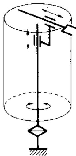
**Fig.5: Workspace of Cylindrical Coordinate Robot.**
