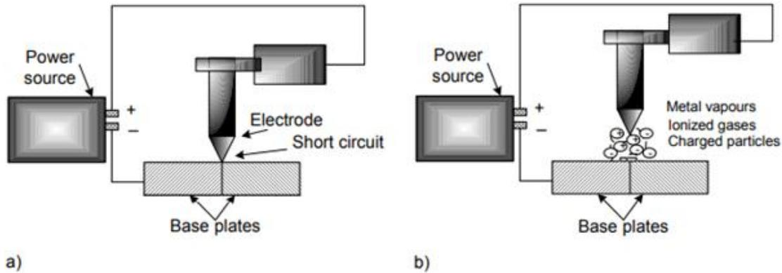
Fig. 4.3 Schematic diagram showing mechanism of arc initiation by touch start method a) when circuit closed by touching electrode with work piece b) emission of electrode on putting them apart
