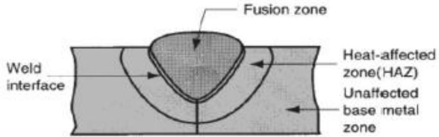
Fig. 4.2 different zones in fusion welding
