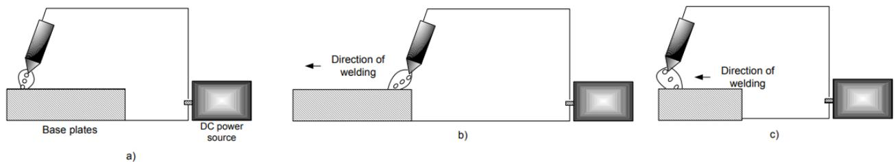
Fig. 4.6 Schematic diagram showing welding a) without arc blow, b) with forward arc blow and c) with backward arc blow
