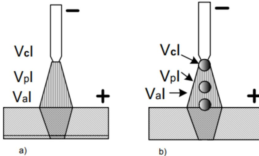
Fig.4.8 Schematic of heat generation in different zones of the arc of a) nonconsumable arc and b) consumable arc welding processes.
