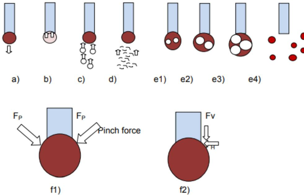
Fig.4.5 Schematic diagram showing different arc forces a) gravitational force, b) surface tension force, c) force due to impact of charge particles, d) force due to metal vapours, e1 to e5) stages in force generation due to gas eruption and f1&f2) electromagnetic pinch force
