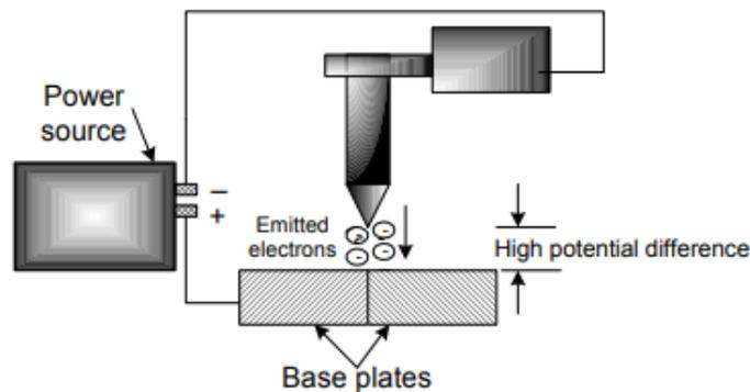
Fig. 4.4 Schematic diagram showing the field-start method of arc initiation
