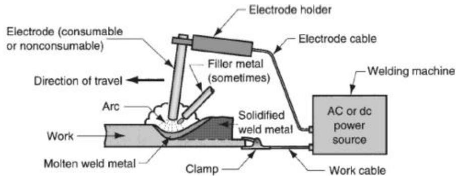
Fig. 4.1 Schematic view of an arc welding setup
