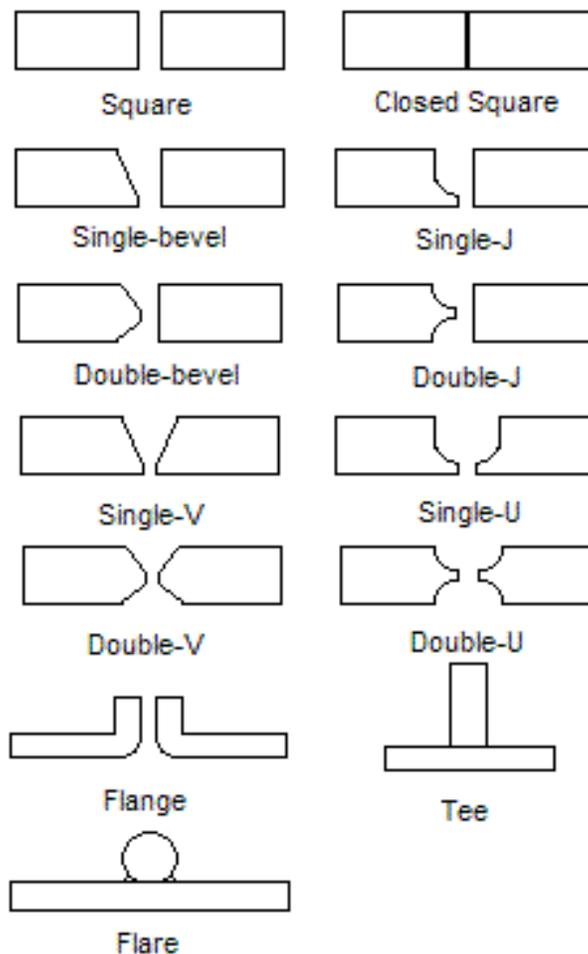
Fig. 4.3 Shape of different weld face
