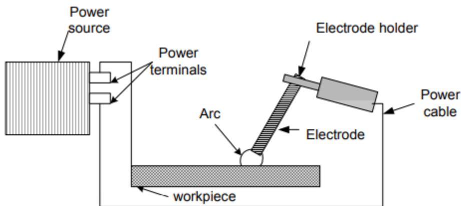
Fig. 4.9 Schematic diagram showing various elements of SMA welding system
