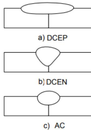
Fig. Schematic diagram showing effect of welding current and polarity
