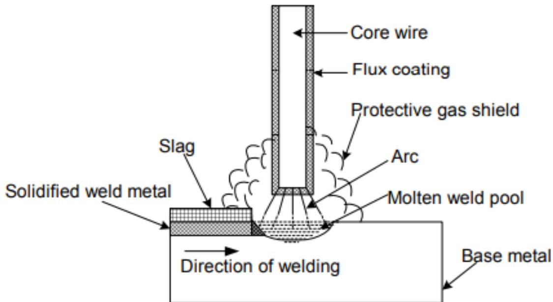
Fig. 4.10 Schematic diagram showing constituents of SMAW
