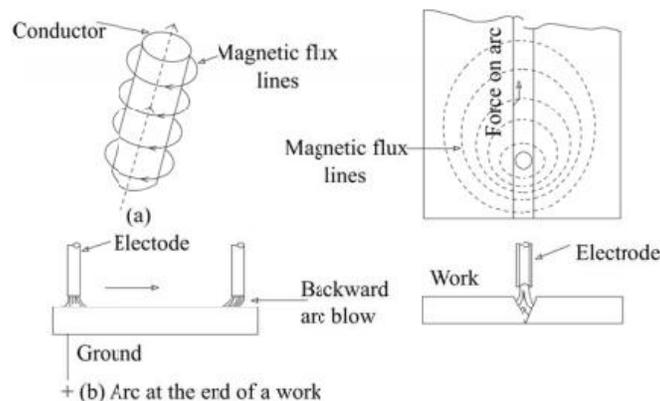
Fig. Schematic diagrams showing generation of electromagnetic force around the welding arc & electrode causing arc blow
