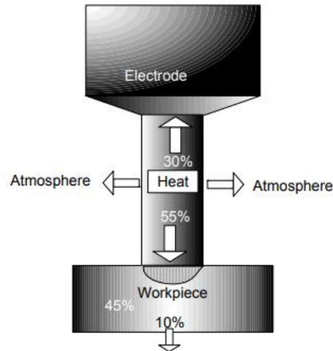
Fig. 4.7 Distribution of heat from the welding arc in DCEN polarity
