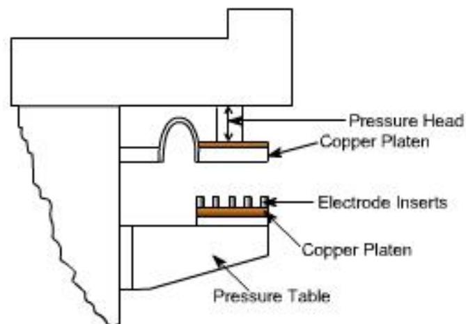
**Fig 5.7 Resistance Projection Welding Machine**
