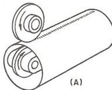
**Fig 5.5 Process of Seam welding**
