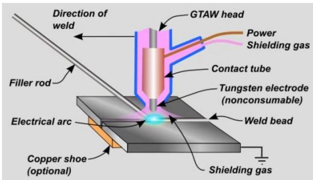
Fig.5.1 Schematic of tungsten inert gas welding process
