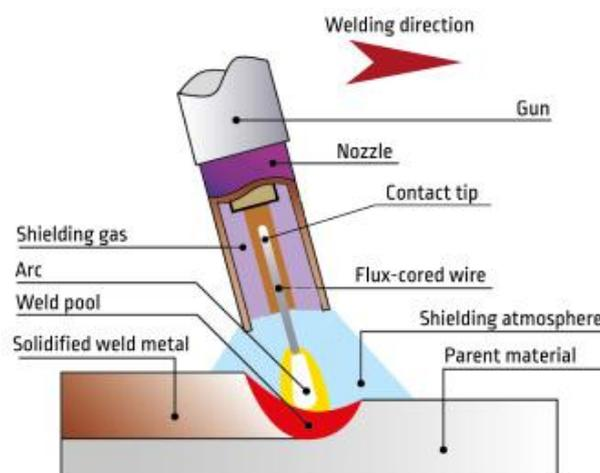
Fig.5.2 Schematic of GMAW process
