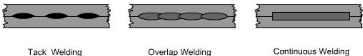
**Fig 5.6 Type of Seam Welds**
