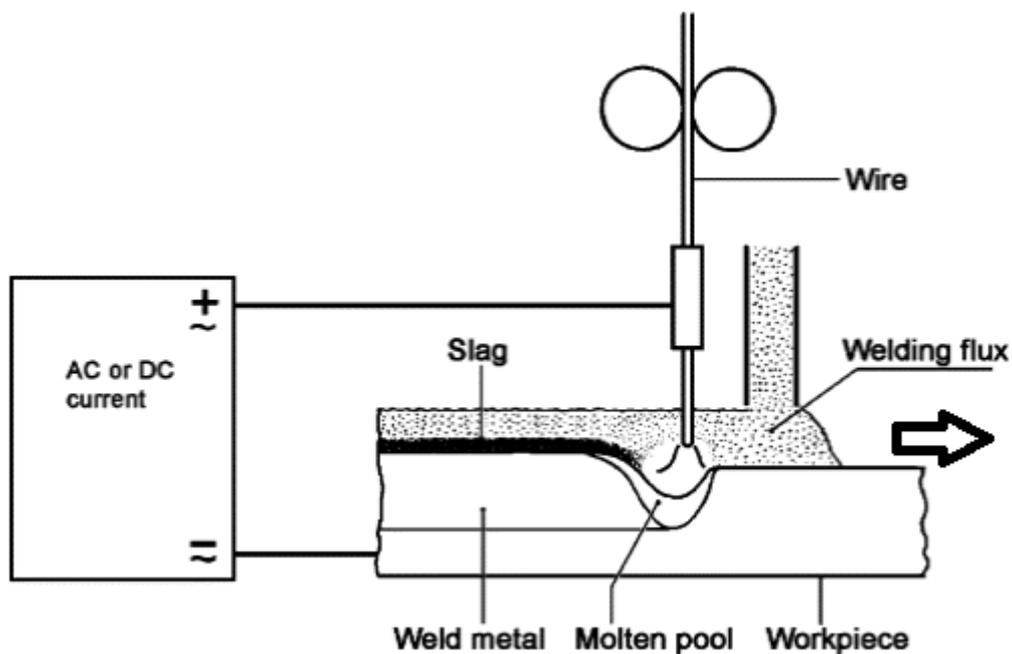
Fig.5.3 Schematic of Submerged arc welding process
