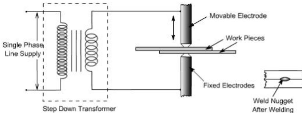
**Fig 5.4 Principle of Resistance spot Welding**
