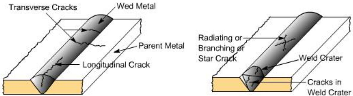
**Fig 5.9 Various Types of Cracks in Welds**
