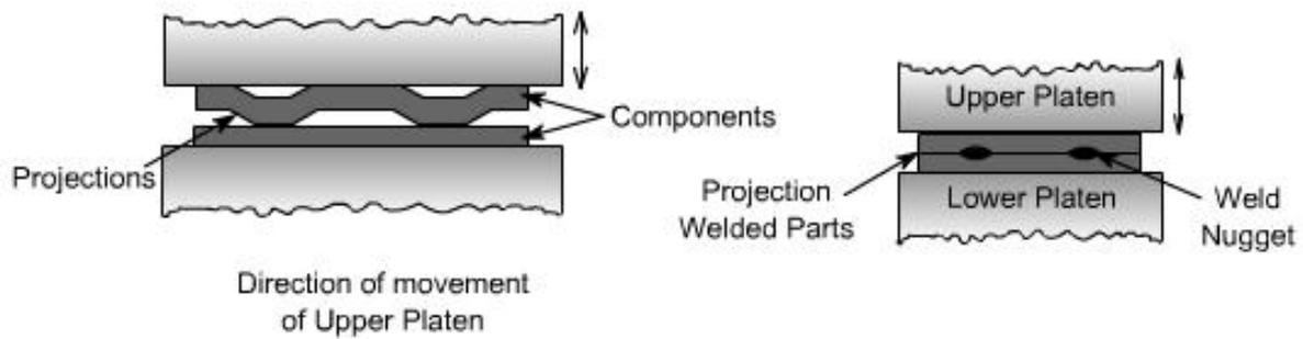
**Fig 5.8 Formation of Welds from Projections on Components**
